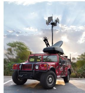
*xMax expeditionary comms. system deployed in a mobile command vehicle.*
